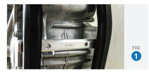
Locate the skid plate and 24-016-02 clamp onto the rear cross member of the frame [Fig. 3]
